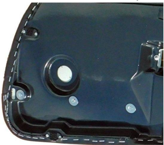
23. Clean the door Velcro clips by running an Exacto blade or small screwdriver between all the rows. Pieces of the mating clips from the old door panel can be trapped and prevent attachment. Remove any stalks that are bent or broken with needle-nose pliers.
