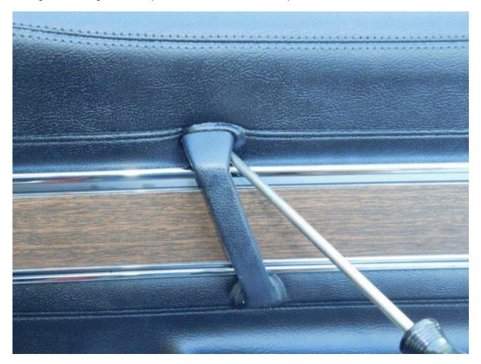
26. Pop the clip into the recess in the door and then install its screw. Hold the door and hit the door panel at the location of each Velcro clip to attach them.
