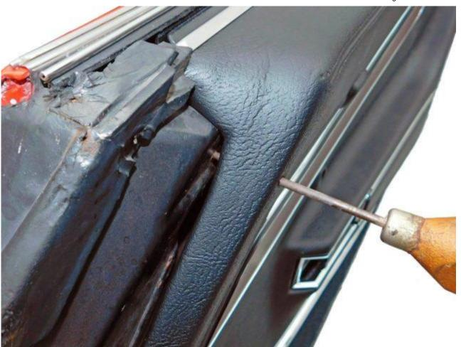
21. Elongate the door pull hole in the C3 Corvette door panel backing until the screw hole in the door is accessible. Tip: a Dremel tool with a side cutter (multi-purpose) bit makes this easy.
