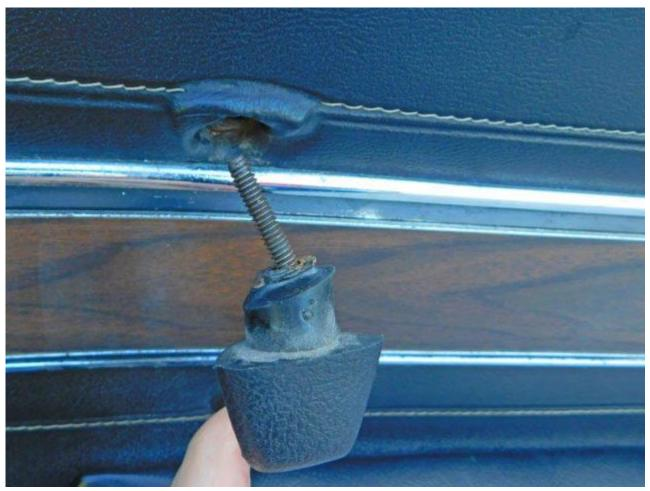
9. Remove the two metal clips located near the lower front and lower rear of the C3 Corvette door panel. Remove the window crank clip, handle and spacer if so equipped.
