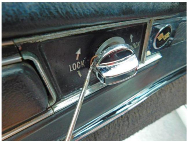
7. Remove the door release handle. Pull the handle out to access and remove the one Phillips screw that attaches it. Hold the door handle in the open position and pull it forward to slide it out.
