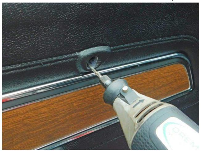
22. Make an imprint on the exposed door panel foam by firmly pressing the door panel against the window regulator shaft. When the panel is removed, cut the foam and vinyl at the imprint. (This is not necessary for cars with power windows.)
