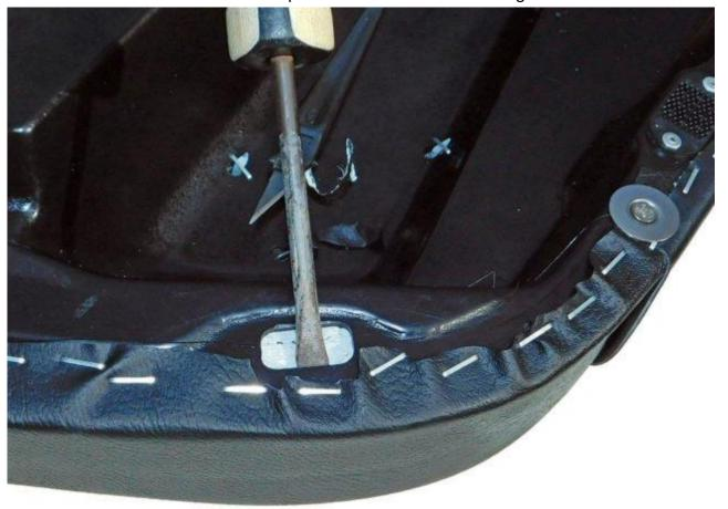
16. Remove a portion of a staple if necessary to get the clip to slide all the way out on the door panel. Cut the staple with wire cutters and remove just one side of the staple if that's all that's needed.
