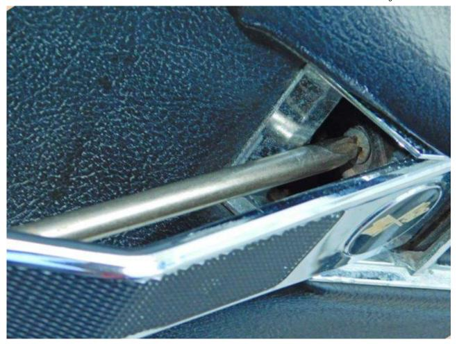
8. Remove the two door pull screws. Tip: use a good #2 Phillips screwdriver and make sure that its tip squarely engages each screw. These are machine screws and may require some force to break them loose and remove them. Be careful: rounding this screw head will create much more work.
