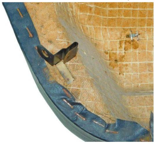
15. Insert a flat blade screwdriver under the plastic backing on the new panel to break the foam adhesive loose to enable the clip to slide between the backing and the foam.
