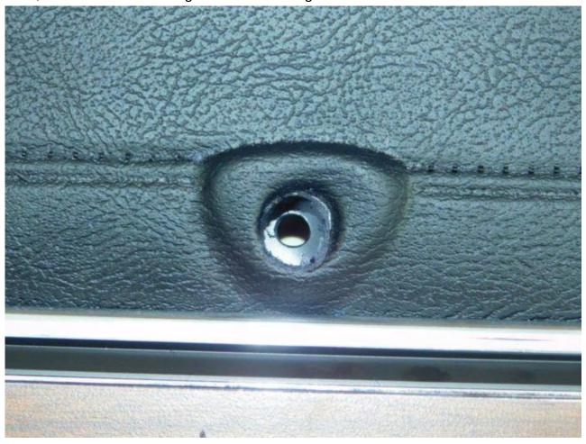
13. Punch a hole through the vinyl at the location of the two screws on the top of the door panel. Heating the tip of an ice pick forms a good hole that is less likely to tear. Insert the pick from the backside through the center of the metal ferrule.
