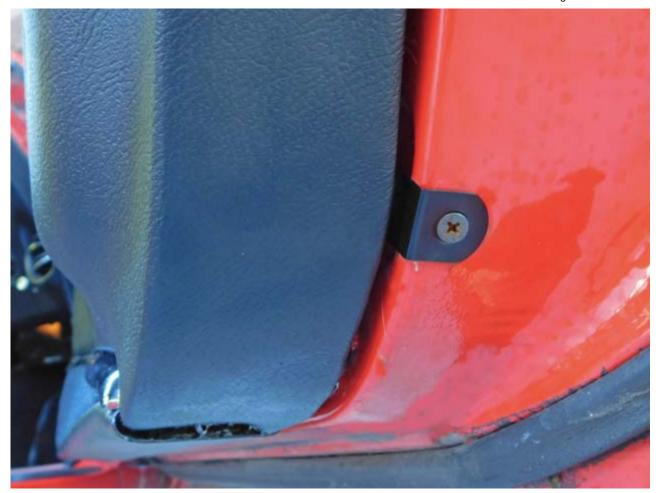
27. The old Velcro clips on the door might not hold onto the door panel Velcro clips. Corvette Central offers new Velcro clips (part number 483311 (https://www.corvettecentral.com/c3-68-82/tops/t-top-headliner-moulding/68-82-door-panel-ttop-headliner-velcro-fasteners-483311? returnurl=%2fsearch%3fcurrentsearchcategoryid%3d%26q%3d483311)) that can be popriveted to the door.
