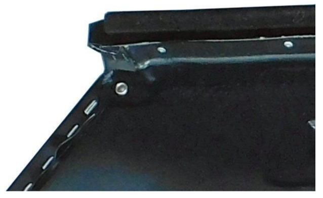
**14. Remove both metal clips** from the old door panel. It is not uncommon for this area to break on older door panels and no longer hold the clip. The plastic backing of the new door panels should be more durable. New clips are available from Corvette Central (part number 483310 (https://www.corvettecentral.com/c3-68-82/interior-trim/door-panel-trim/68-77-doorpanel-mounting-metal-clips-with-screws-483310)).
