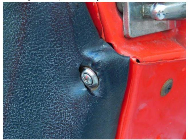
3. Electrical tape can only do so much to cover up the cracked vinyl. Above those cracks, large splits in the armrest area were effectively concealed for years by armrest patch panels. Corvette Central offers the patch panels in correct factory colors for <u>1969-77 door panels</u>.
