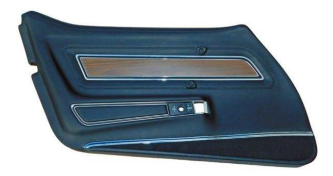
5. The replacement door panels have a plastic backing. The backing of the older panel was a fiberboard material. As the vinyl shrank over time, the older door panel warped causing the lower portion to curl away from the door.
