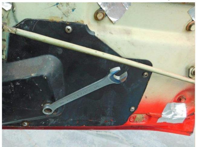
19. Bend the flanges on the top of the door if necessary for the new door panel to slide over the outside of this metal. Install the new door panel over the top of the door for a test-fit. It may be necessary to tip the bottom of the door panel away from the door and push the top outward.
