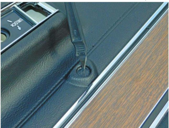
12. Drill a 1/4 inch hole in the center of the newly opened-up door pull hole. Later, during the test-fit, a Dremel tool will elongate this hole to align with the screw hole in the door.
